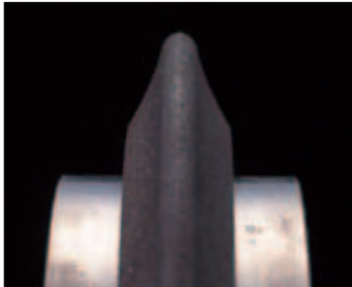
Profile of electroplated CBN-forming wheel
