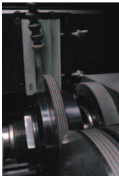
Crush roll forming by metal bond wheel "FX-350"
