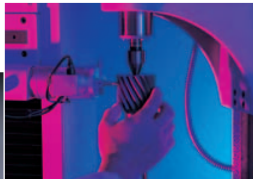
Gear dresser form accuracy being measured
